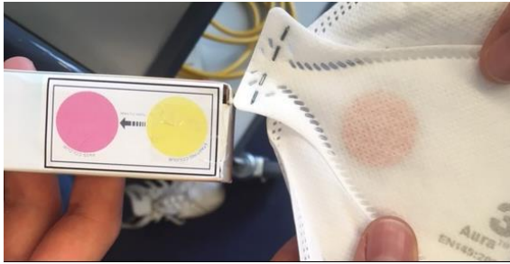
Figure 1. UV detection strips with color coding. Yellow for exposure, discoloration after detection to pink
